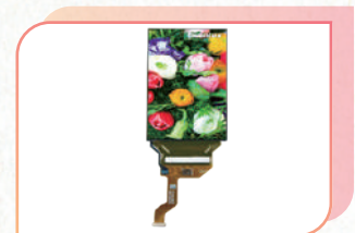
Innolux Corporation-LCD with invisible camera
