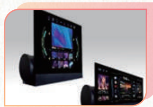
AUO Corporation-14.6-inch Rollable Micro LED display
